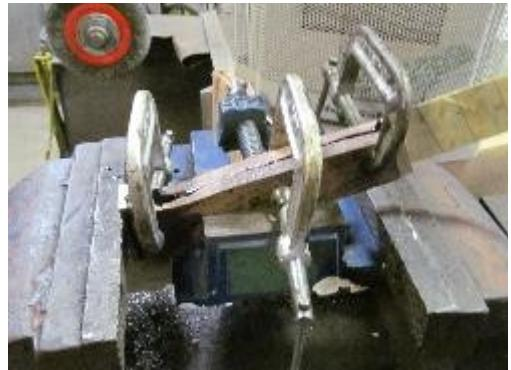
The next step is to insert the 1/8" pins and jazz the handle up with mosaic pins. The tooling needed is shown here = a drill the size of the mosaic pin to be used (#2 at 0.221" – and I don't remember where I got 5.6mm tubing to make the pins), a depth indicator, a saw jig and the Allen wrench needed for the jig.
