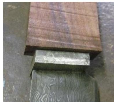
The next step is to etch-a-sketch the recess into the thicker block. A bit of white-out makes seeing the scribed outline of the tang a whole lot easier. Incidentally, white-out is removed by acetone.
