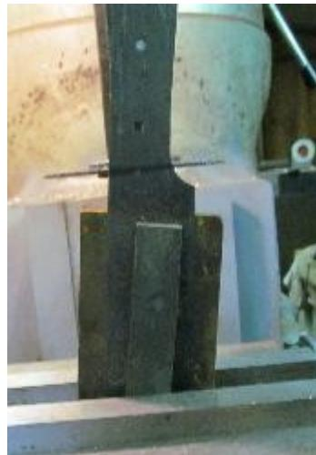
The blade was positioned at a slight angle (because I think it just looks cooler!) and the saw was moved to the left and positioned with the axis of rotation of the saw perpendicular to the tang's dorsal surface (ok – the spine...whatever). The mill was SLOWLY cranked to the left and to create an approximately  $\frac{3}{16}$ " slot.
