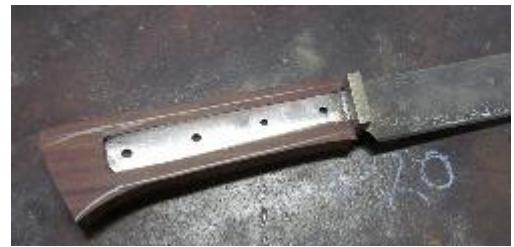
When that was done, the tang was glued into the recess using 5-minute epoxy and black colorant. Note the masking tape protecting the blade.
