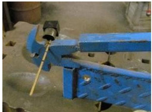
All the pins are gently started in their respective locations and then epoxy is smeared over the sides as well as into the cavities for the 1/8" pins on the opposite scale.
