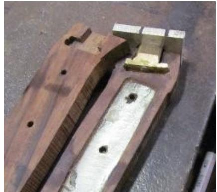
The solution is shown here. Use a small drill press vise (2.5") to hold the pommel perpendicular to the vise's jaws. The whole assembly is then place in a machinist vise and the pommel is pressed to the mating surface. Once the epoxy sets up inside the pommel recesses, there is no way anything can come loose without destroying the handle first.
