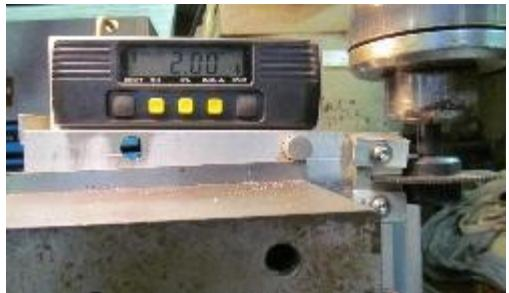
The table is cranked to the right by the depth of the slot (in this case, 0.767"). The saw is withdrawn and the jig is cranked up to the same angle on the other side of dead level. The table is then adjusted so the cut will form the other side of the slot taking into consideration the 0.080" thickness of the saw. Depending on whether the slot widens or narrows to the left, you'll have to do some thinking.
