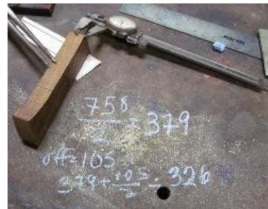
A line was drawn on the block at that offset and the block was cut on the band saw. Note that the spine of the block was left square to make the sawing easier. Eventually the "ski jump" curve shown here will be echoed on the spine side.
