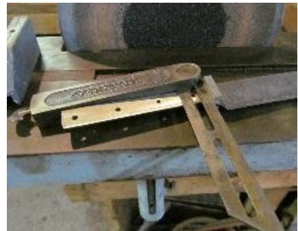
Once the angle is set, the guide on the disk sander can be set to the same angle.
