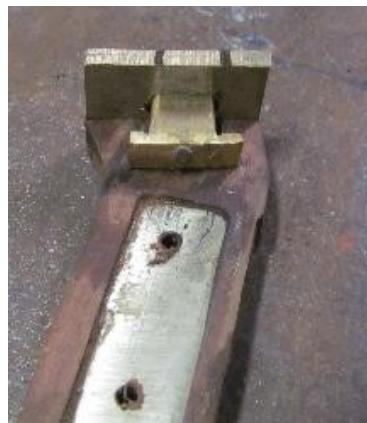
Recesses were made in both scales. It's finally time to glue everything together. The pommel recesses were filled with epoxy and more epoxy was spread over all the mating surfaces. Using alignment pins makes the assembly fairly easy and the scales were clamped with several “C” clamps. The only major question left is how to press the pommel firmly against the mating surface since the pommel and the guard are not parallel to one another.
