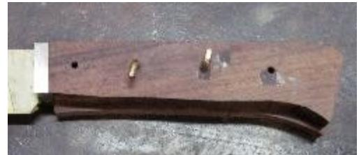
When clamped and with the alignment pins in place, the rear surface was sanded smooth and perpendicular to the sides using the disk sander. The surface shown here will be the mating surface to the pommel.
