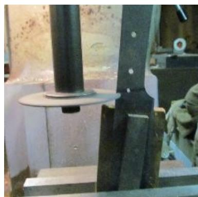
The saw was then repositioned to the right and the second cut was made. The mill table elevation was decreased by 0.25" because the guard material is that thick. The guard will be a "U" shaped block of nickel silver with the bottom of the "U" at the dorsal surface of the tang. The slots are absolutely parallel to one another and 0.25" apart. This same operation could have been done with a carbide slitting saw but at about 100 times the cost.
