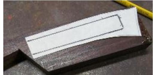
The idea is to split the block taking into account the offset due to the tang thickness (here 0.105"). Given a block of 0.758", the midpoint would be 0.379". Move that 0.105/2" to one side and the thickness of the two scales is known.
